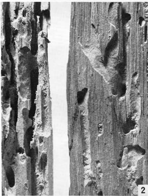
Fig. 1. Ochrocydus huttoni Pascoe. Larval gallery (left) and pupal cell (right) in Leptospermum scoparium . Fig. 2. Ambeodontus tristis (Fabricius). Larval damage in boards of Dacrydium cupressinum . Fig. 3. Phoracantha semipunctata (Fabricius). Radial galleries in branch of Eucalyptus .
